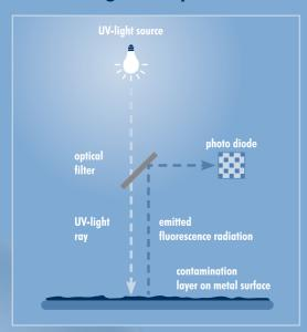
Typical contamination on surfaces in industrial manufacturing processes such as oil, grease, cooling lubricants or parting agents fluoresce when being excited by ultraviolet light. The intensity of the fluorescence increases with the thickness of the contamination.
