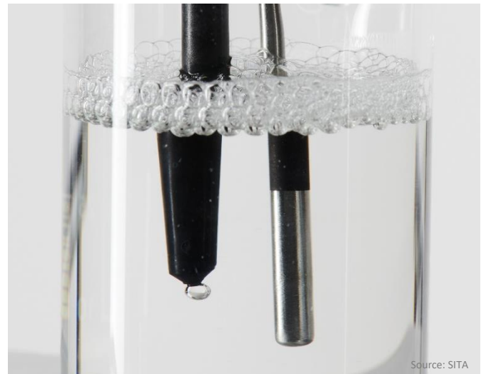
Figure 2: A small air bubble at the capillary tip is used as interface for measuring the dynamic surface tension.
