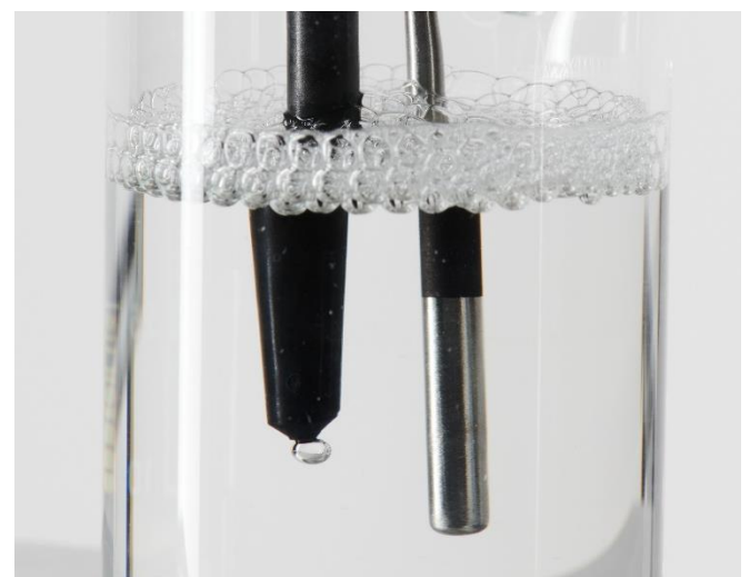
Figure 3: A small air bubble at the capillary tip is used as interface for measuring the dynamic surface tension.
