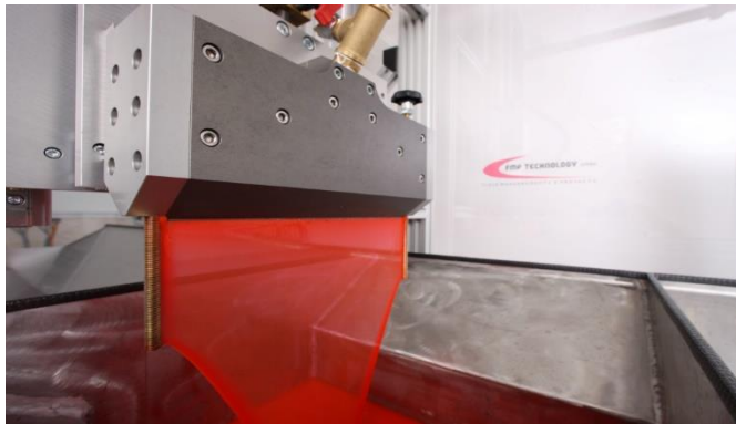
Figure 1: Curtain coating machine
