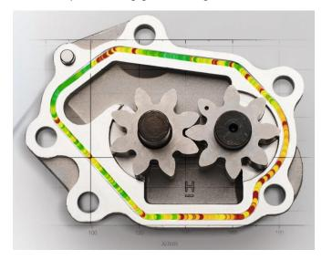
Figure 3: Colour-coded visualisation of the in-line inspection results
