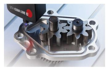
Figure 2: In-line cleanliness inspection of the sealing groove
