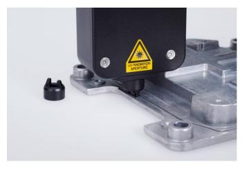
Figure 1: Manual measurement with SITA CleanoSpector and spacer directly on the adhesive groove
