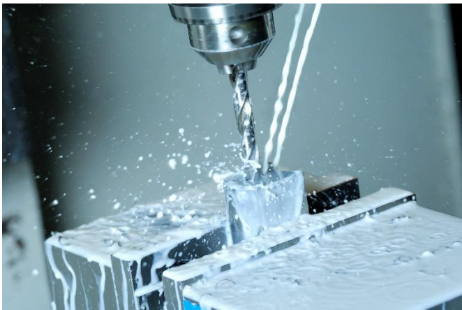
Figure 1: Application of a cooling lubricant during drilling
